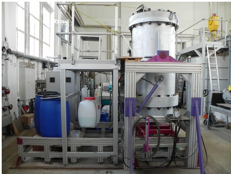
Figure 1.9 Pilot test of sealing elements (actually set up)
