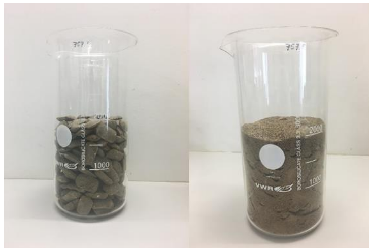
Figure 4.15 Pouring density test; briquette filling (left) and filling with briquettes and granulate (right)
