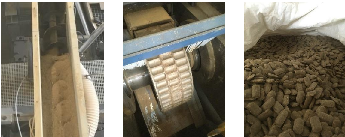
Figure 4.16 Left: feeding material Secursol UHP (G1580) < 3.15 mm; middle: briquetting roller, pocket dimension 3 cm 3 ; right: briquettes ready for shipping in big bags for HTV-6
