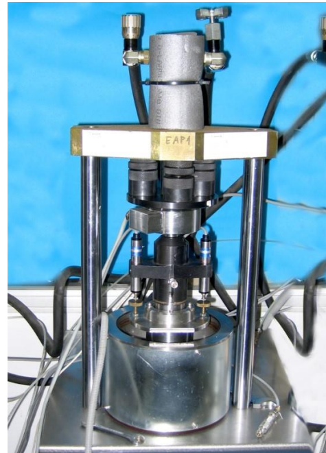
Figure 4.4 Schematic layout and photograph of the high-pressure oedometer equipment
