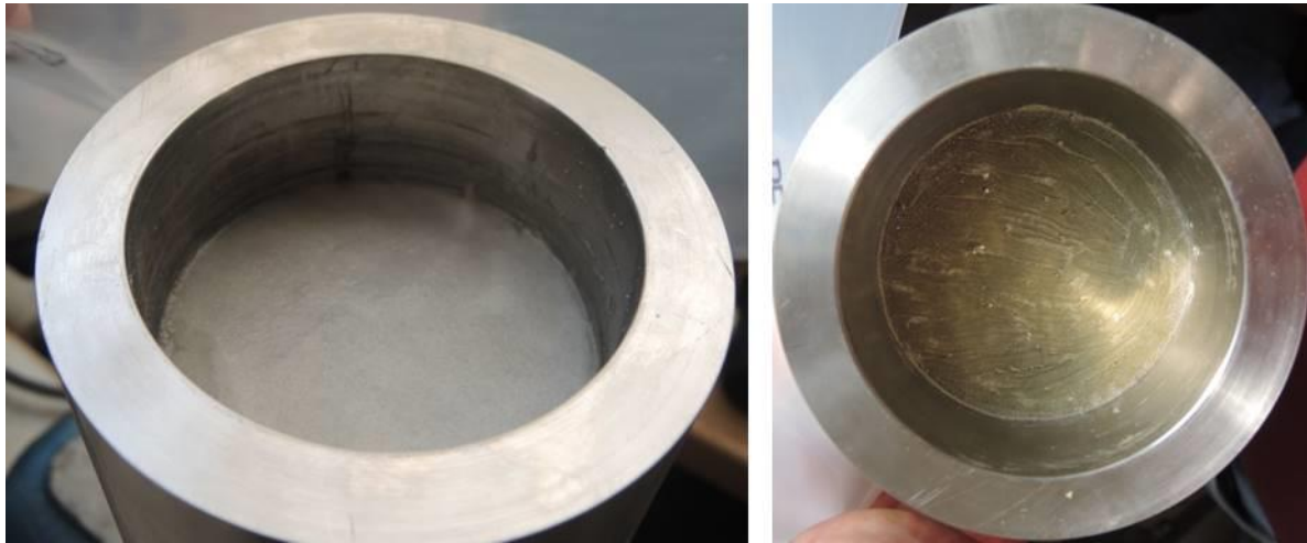
Figure 4.40 Stepwise dismantling of the saturated MiniSandwich specimens: left: wet sand (ES1 Oe7); right: compact bentonite (DS2 Oe8)
