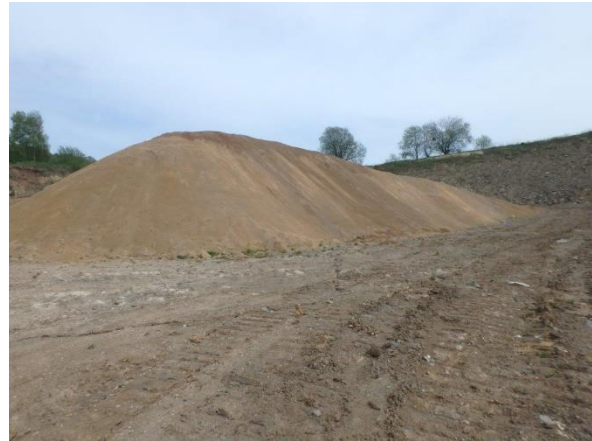
Figure 4.22 30.000 t of mined Secursol UHP, stored in the North of Lower Saxony pit
