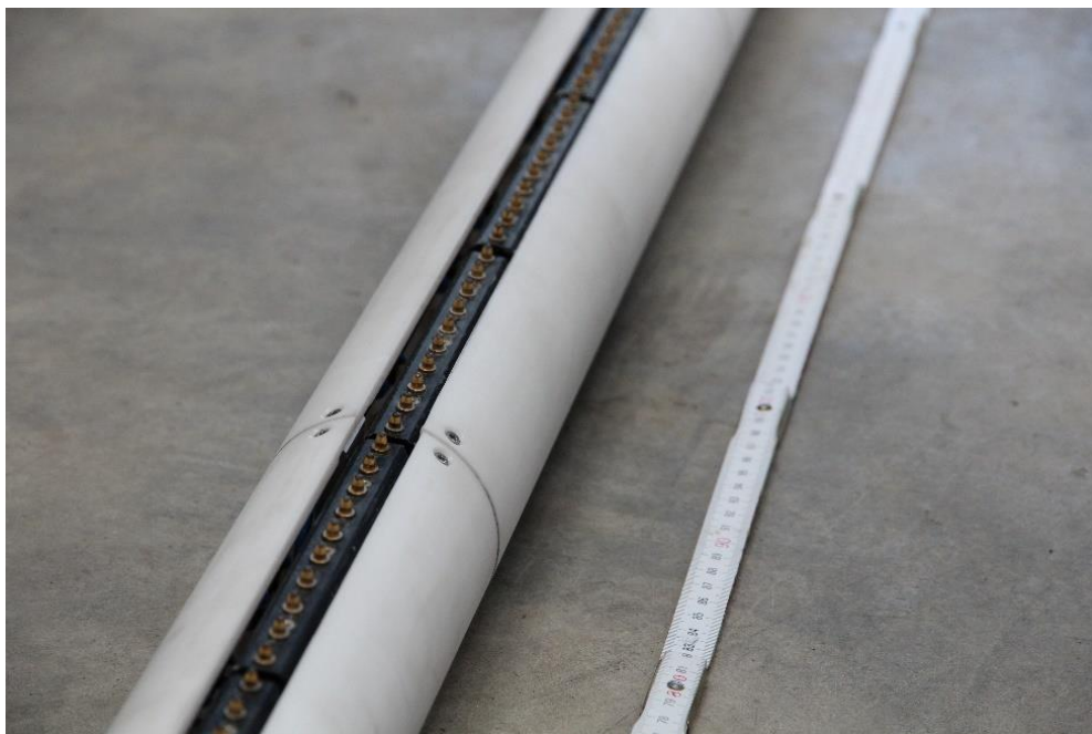
Figure 8.5 Part of the ERT borehole probe GB100-15
