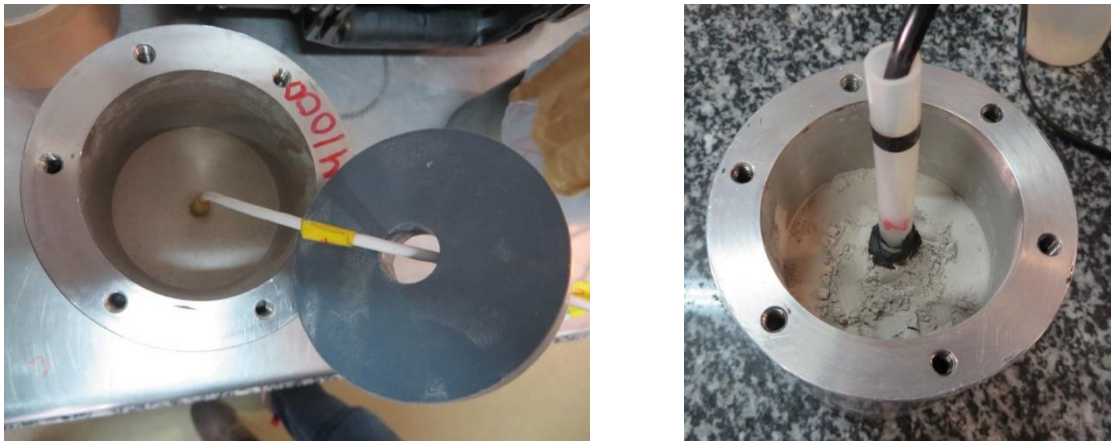
Figure 4.8 Psychrometers (left) and capacitive sensor (right) inserted into the compacted samples
