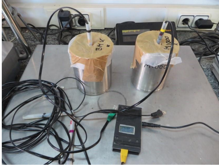
Figure 4.9 Measurement of suction pressure in compacted samples
