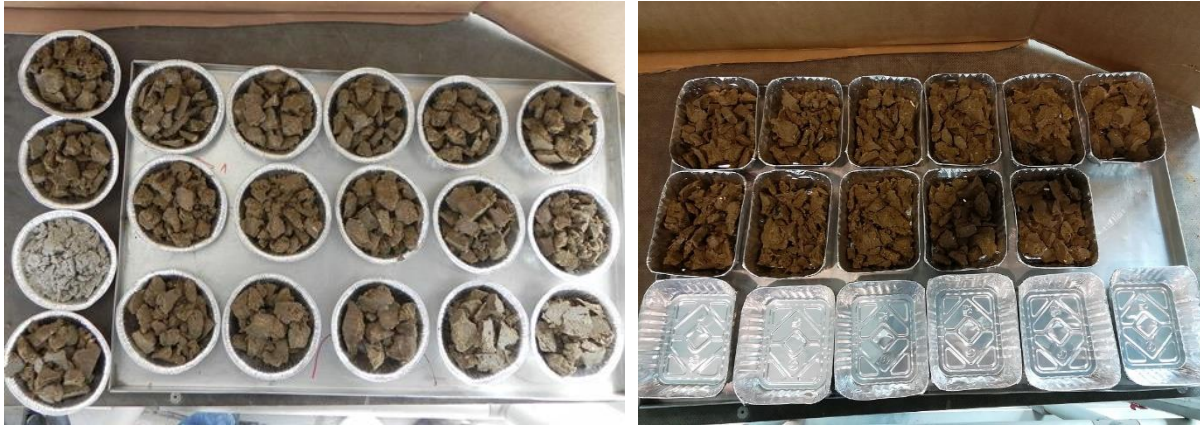
Figure 4.68 HTV-6 Samples for water content measurement
