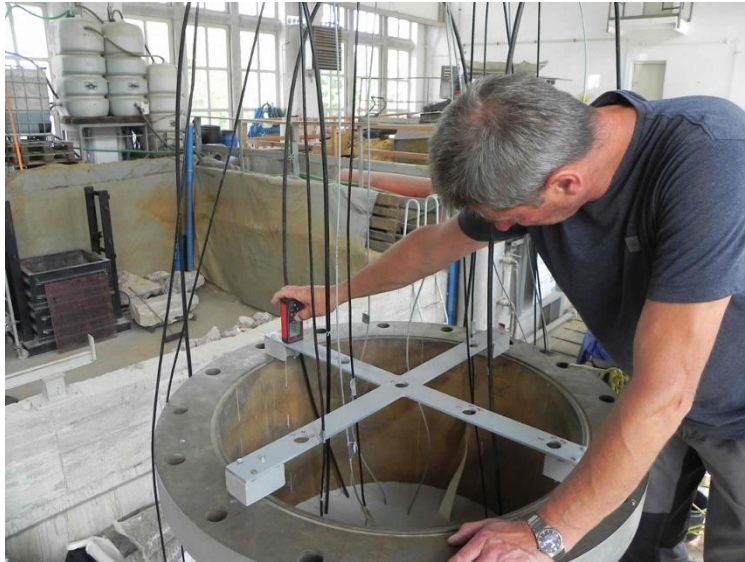
Figure 4.50 HTV-6, ES3 – laser distance measurement
