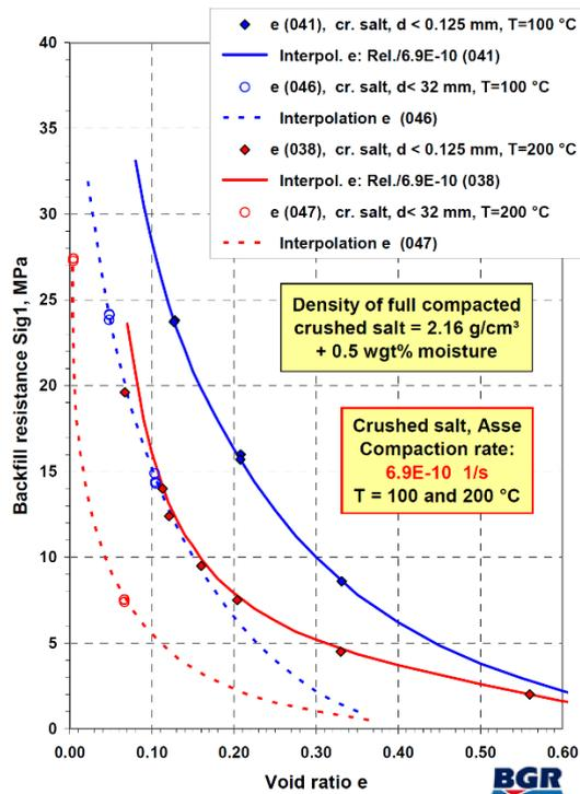
**Fig. 5.4** Influence of the grain-size curve on the Backfill resistance with  $d < 31.5 \text{ mm}$  and  $d < 0.125 \text{ mm}$  /KRÖ 09/
