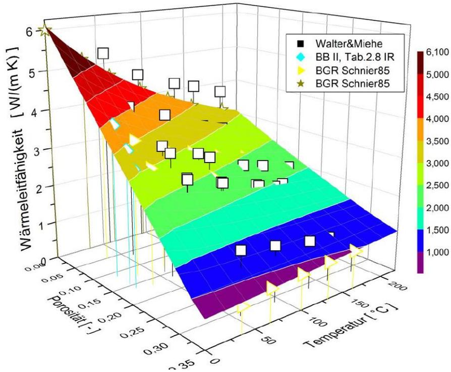
**Fig. 2.4** Heat conductivity of crushed salt as a function of porosity and temperature
