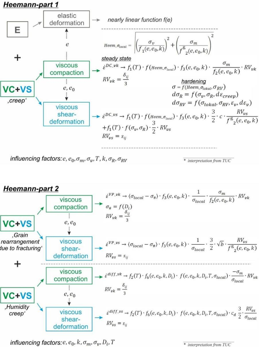
**Fig. 5.22** Structural sketch for the constitutive model Heemann used from BGR
