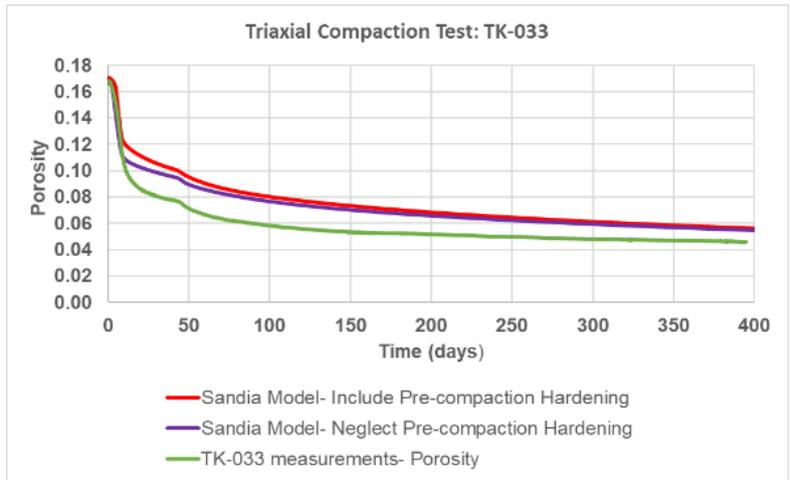
a) Effect of pre-compaction and sample end restraint
