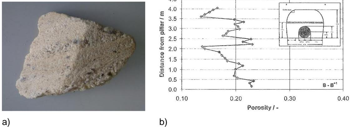
**Fig. 5.5** Distribution of grains: a) Layered structure of backfill material - Sample from the BAMBUS test field /HEE 19/, b) Horizontal porosity distribution in cross section B+1 (1 m behind central plane) /BEC 04/
