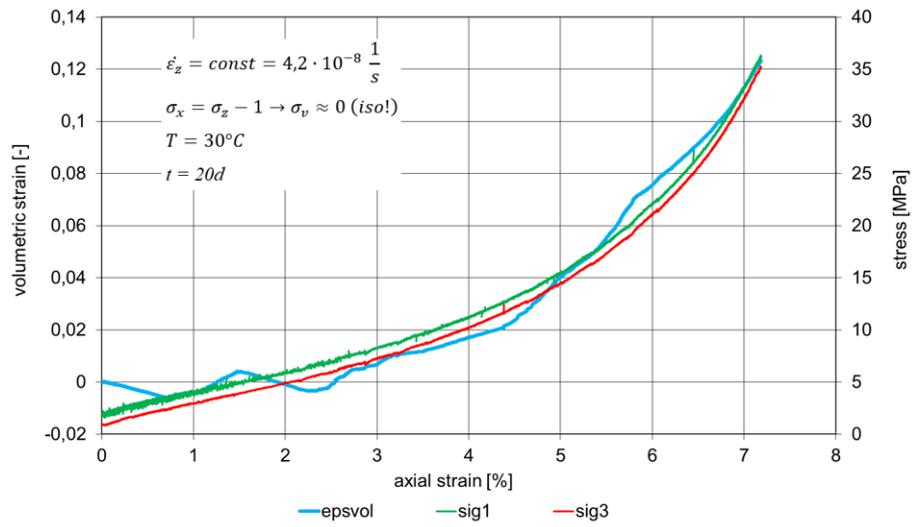
**Fig. 4.65** Results from the TUC-V3 experiment
