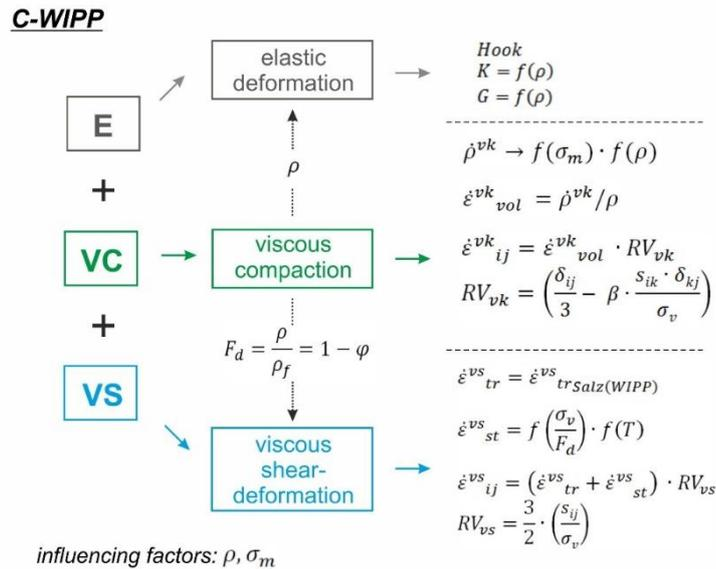
Fig. 5.15 Structural sketch for the constitutive model C-WIPP/Itasca
