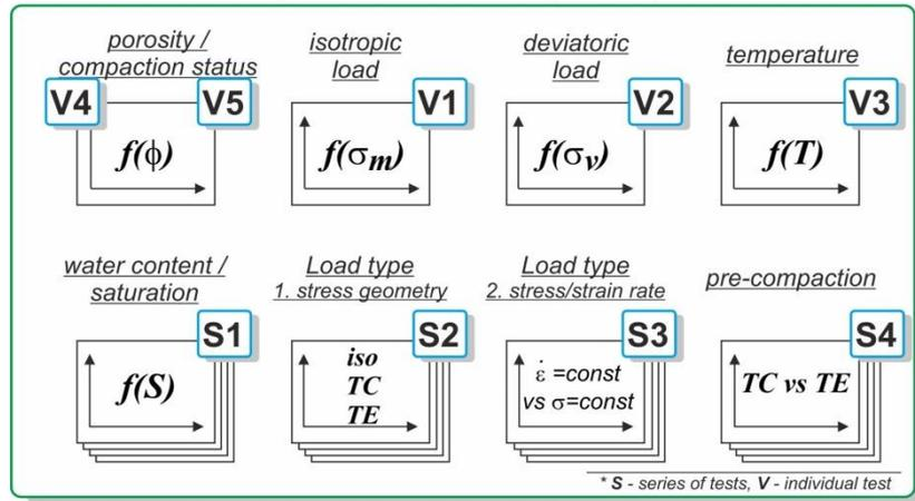
**Fig. 6.6** First iteration step for planning the laboratory test program
