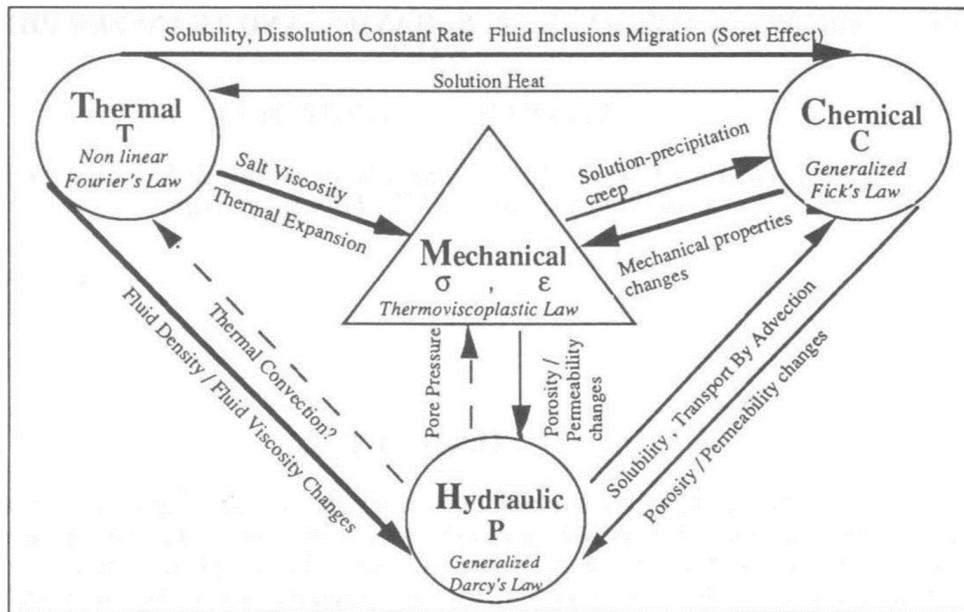
Fig. 5.2 Main coupled processes in salt /COS 93/
