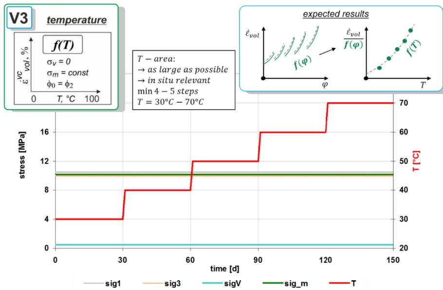
Fig. 6.10 Loading history of test type V3
