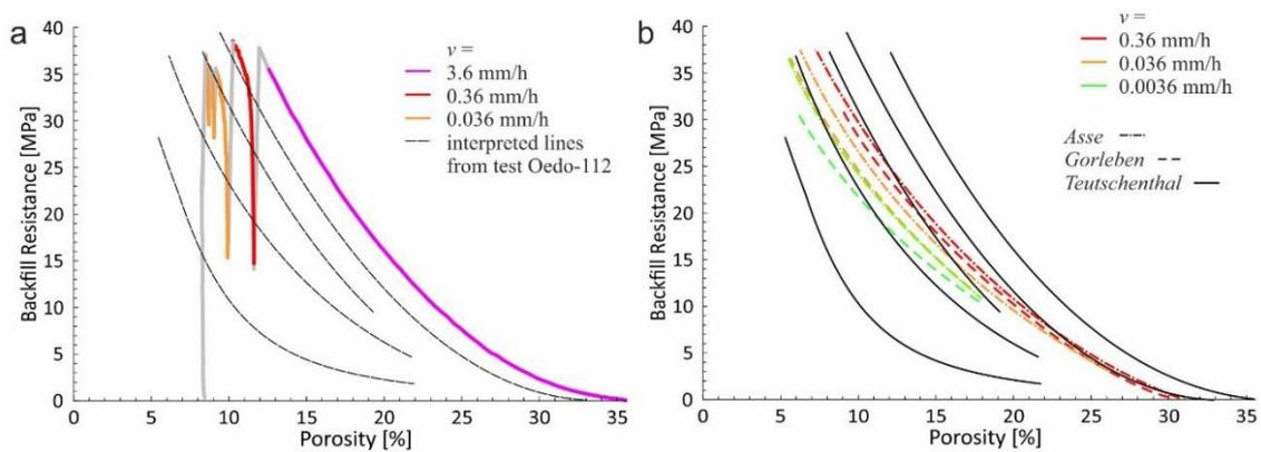
**Fig. 4.13** (a) Load resistance versus porosity values given for differing strain rates (in colour) of test Oedo-113, b) Interpreted lines of crushed Asse and crushed Gorleben salt behaviour at different compaction speeds (in colour) and interpreted lines of Oedo-112 and Oedo-113 (solid black lines)
