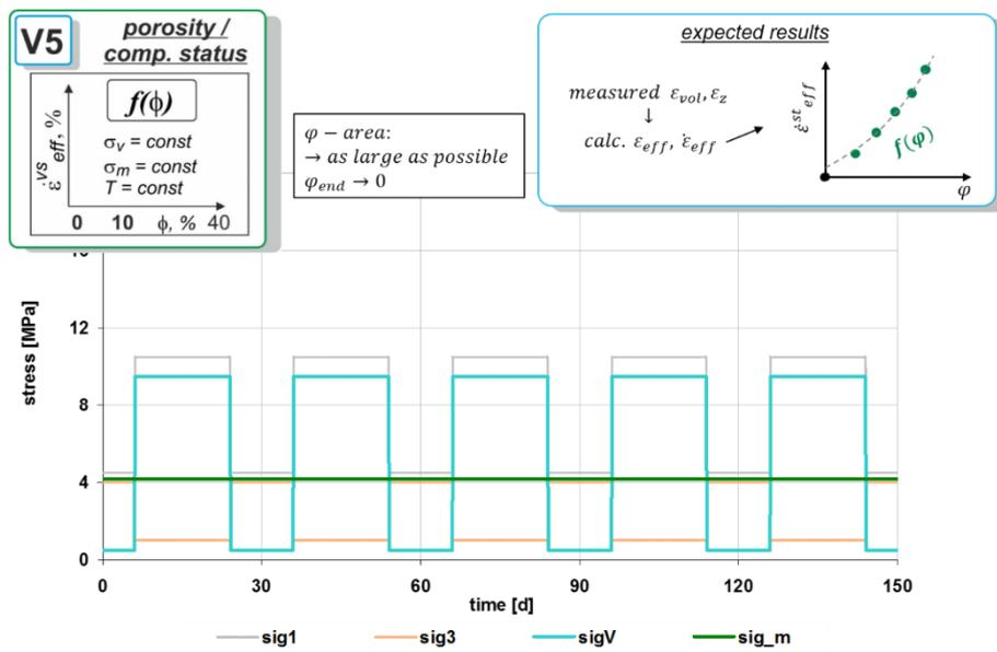
Fig. 6.12 Loading history of test type V5a
