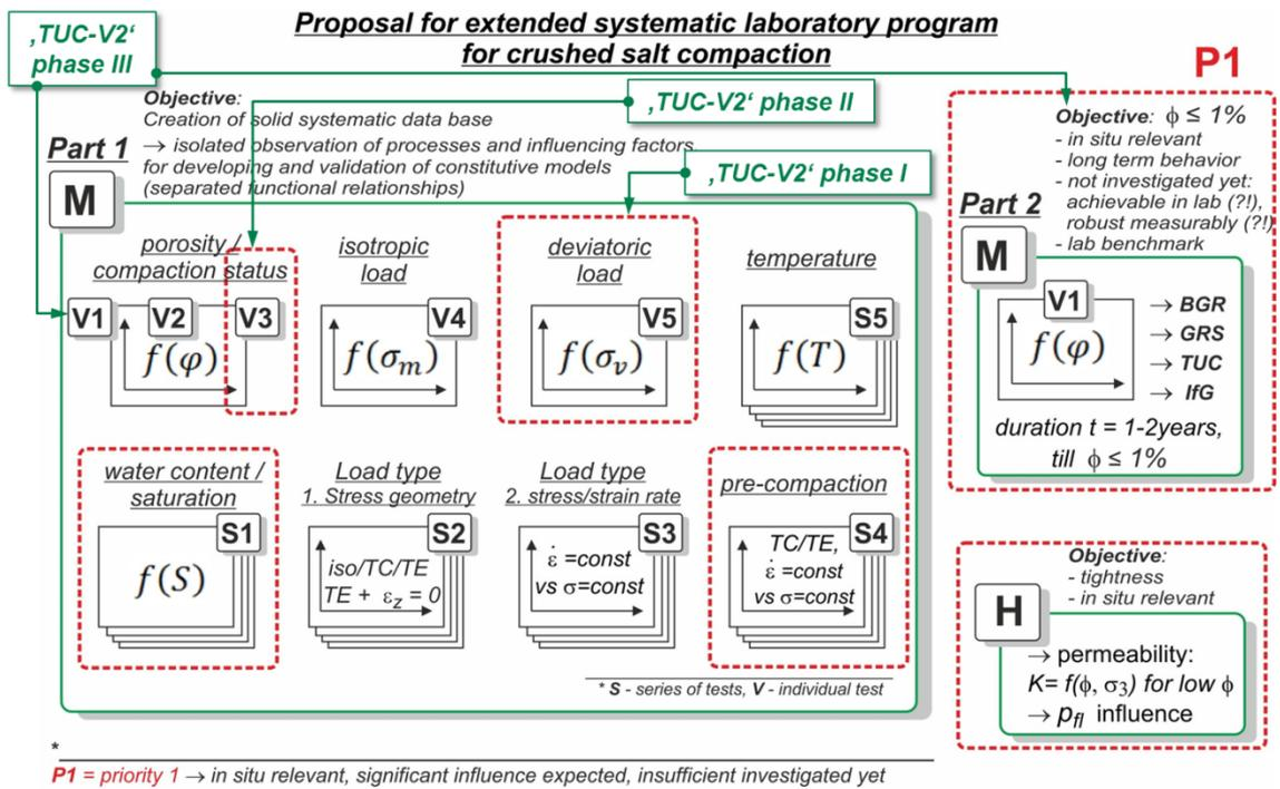
**Fig. 6.19** Final version of the approach for a comprehensive systematically laboratory program with prioritization and allocation of the TUC-V2 test
