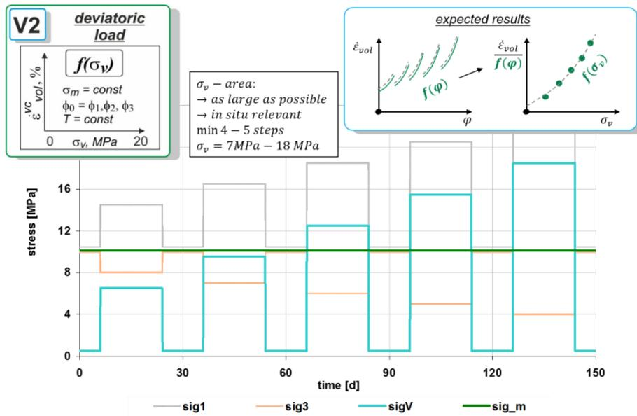
Fig. 6.9 Loading history of test type V2
