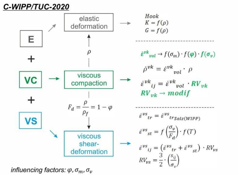
Fig. 5.18 Structural sketch for the constitutive model C-WIPP/TUC
