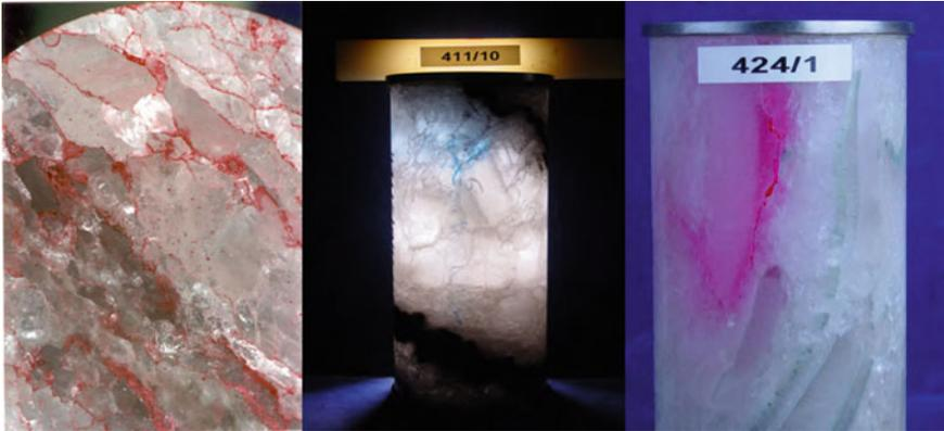
**Fig. 3.1** Percolation of a colored solution on grain boundaries in hydro-mechanically coupled triaxial compression tests on salt specimen
