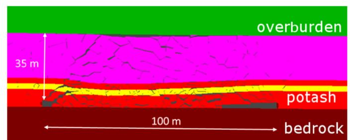
Figure 7: Geomechanical model of disturbances in the hanging wall due to horizontal volume reduction in the potash seam. Note the inclined fracture development.
