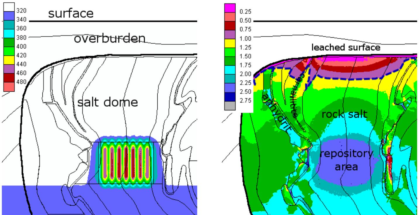
Figure 14: Model of borehole emplacement in the Gorleben salt dome 30 years after emplacement. The figures span  $1400\text{ m} \times 1400\text{ m}$  each. *Left panel:* Temperature in K, *right panel:* ratio of minimal principal stress to groundwater pressure (minimal stress criterion). The criterion is violated for values smaller than one, i.e. purple, red and pink (above blue dashed line).
