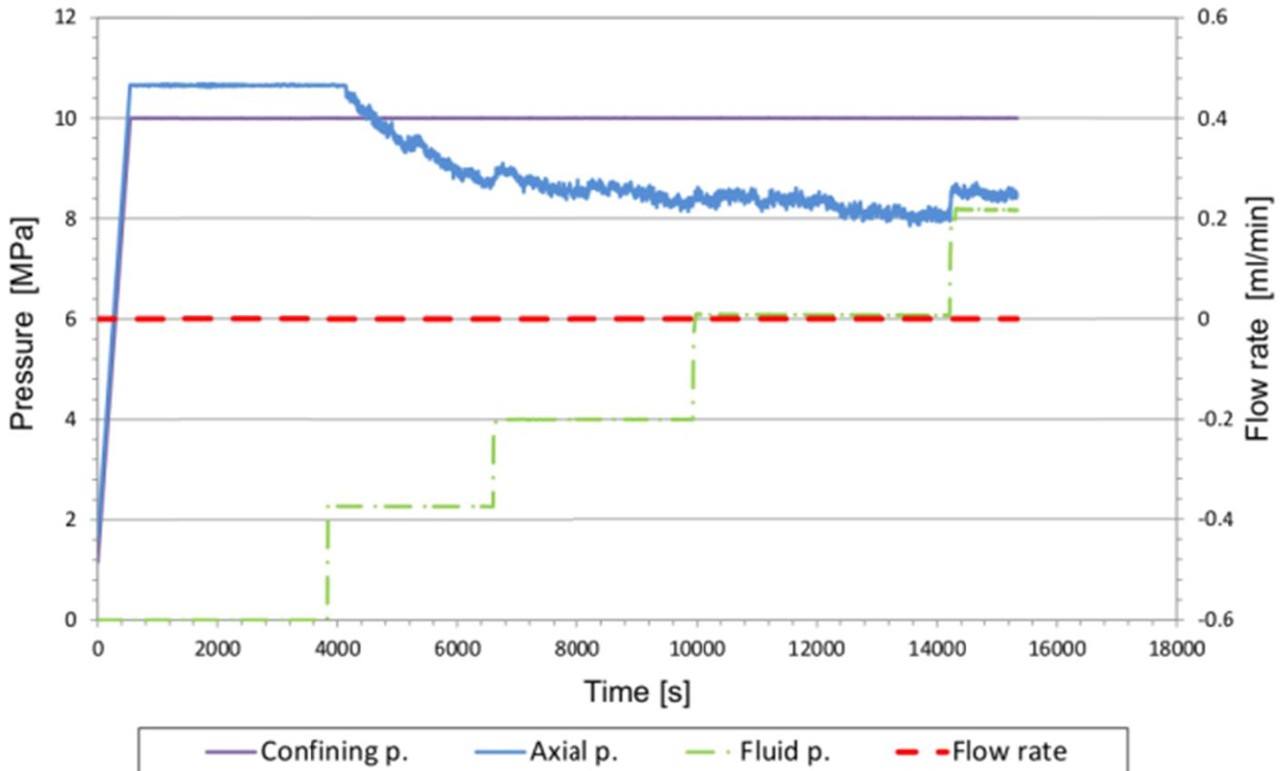
Figure 9. First experimental stage: Pressures and flow rate through the sample versus time. After about 4000 s, the experiment is switched to strain control with constant confining pressure, hence the axial pressure shows small wiggles. The fluid pressure is increased in steps of 2 MPa. No fluid flow could be observed.
