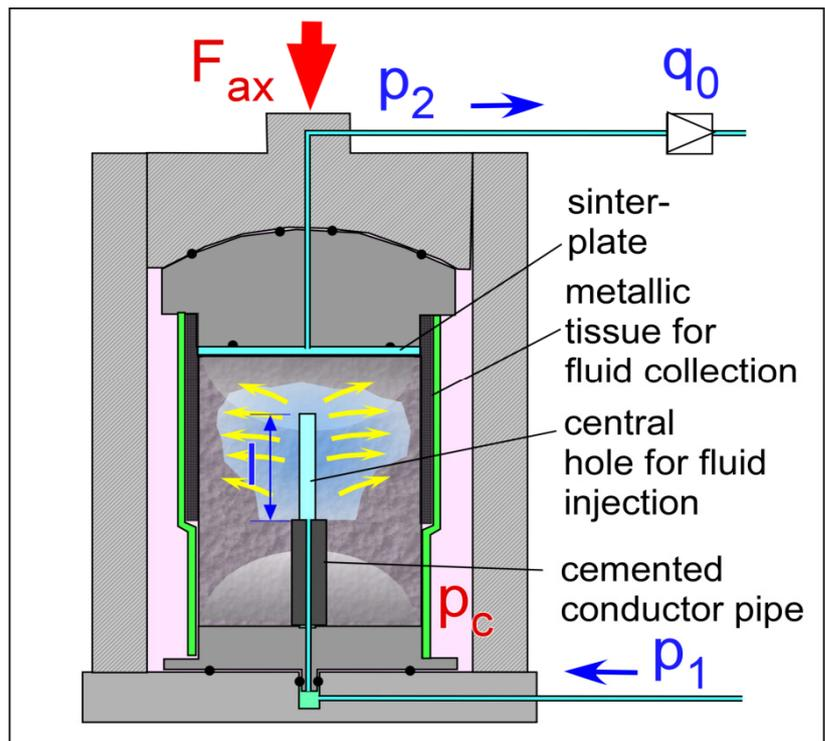
Figure 8: Servohydraulic testing machine and experimental setup for permeability measurements. Flow rates are measured at the top (labelled by  $q_0$ ).
