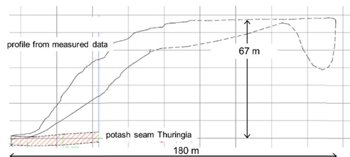
Figure 6: Geometry of the tertiary CO<sub>2</sub> cavern in the middle Werra rock salt above the potash seam Thuringia.
