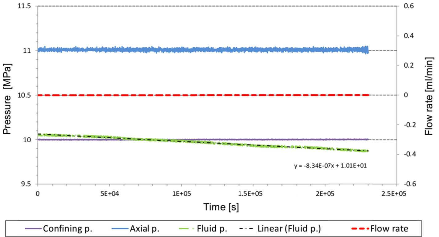
Figure 10. Second experimental stage: Axial and confining pressure are kept constant at 11 and 10 MPa, respectively, with fluid pressure at 10 MPa. Again no fluid flow through the salt is observed. Fluid pressure decreases very slowly, probably due to diffusion into the sample.
