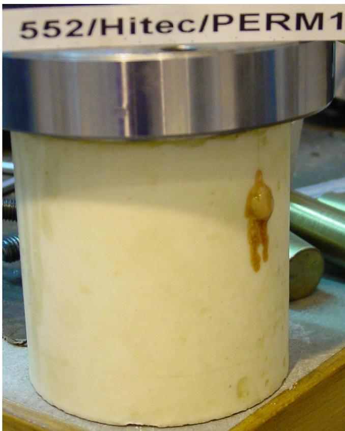
Figure 12. HITEC sample after percolation test, with the fluid indicated by the tracer and bubble. The leakage is localised to a small spot.
