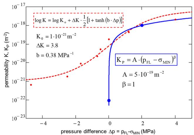
Figure 13: Permeability of rock salt (red, dashed) and HITEC (blue, solid). The power-law behaviour is predicted by fluid percolation models.
