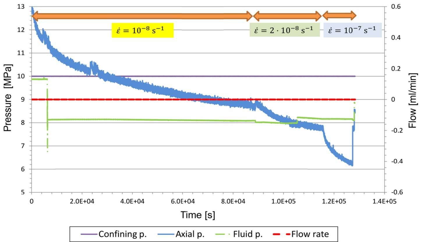
Figure 11. Third experimental stage: The sample is extended at increasing rates, until axial pressure drops sufficiently below fluid pressure for rapid percolation to develop.
