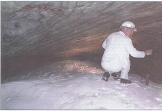
Figure 3: CO<sub>2</sub> glacier after an underground gas blow-out in rock salt (CO<sub>2</sub> becomes solid below -70°C).
