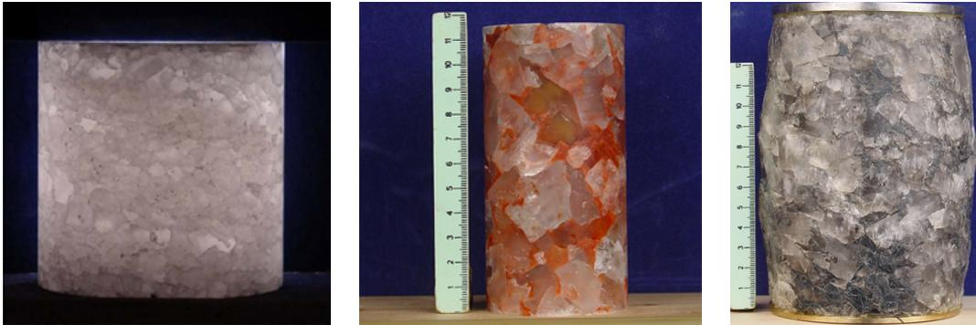
**Fig. 11.1:** Samples of rock salt with clearly visible grain structure.
