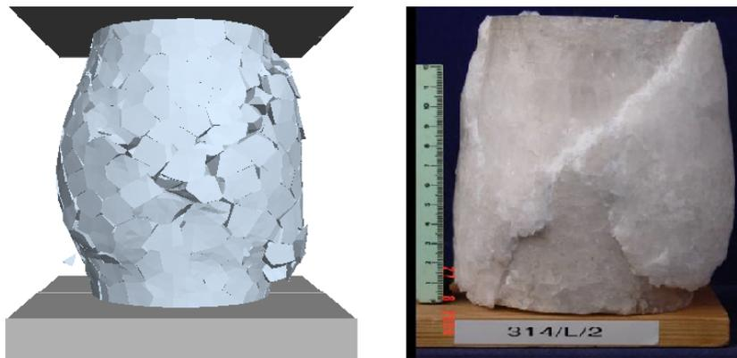
**Fig. 11.6:** Deformed discontinuum-mechanical model of a rock salt sample after testing (left) in comparison with the real specimen (right).
